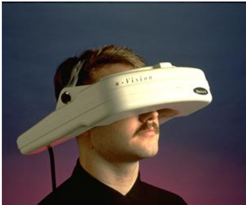
A helmet-mounted display from n-Vision, Inc. The SynchroMaster 100HD provides the color field sequential signal for its miniature CRTs.
