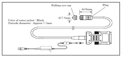
For applications where the detachable-end feature is not required, XtendView Plug & Play cables offer a lower cost solution with the same high quality performance. Details available on separate brochure.
